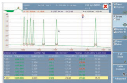
Graphical and tabular display showing pass/fail indicators and out-of-range values
